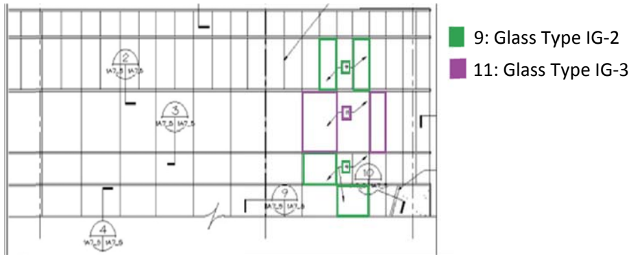
Figure 8: Partial Elevation | Glazing
